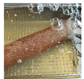
Ultrasonic Cleaning of Steam Filters
